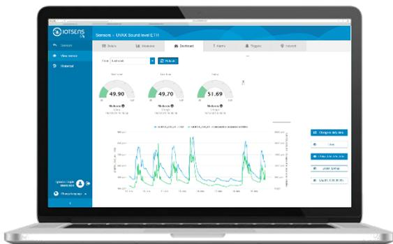
Through the integration of this sensor in the IoTsens Cloud platform, the software offers the hourly and daily data of these variables, as well as their corresponding calculations to know if the levels comply with the regulation.
